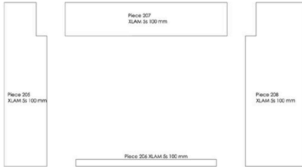
External view - Explose of Xlam Panels
