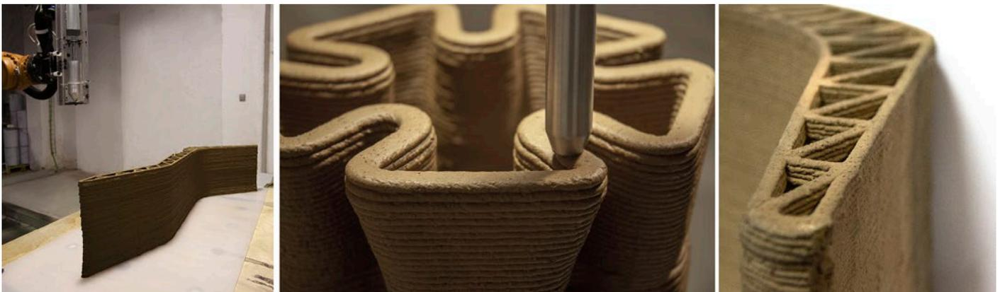
subset. The ALM tools are mainly two: powder-bed deposition (3D printing), and cold extrusion (3D plotting), to be used differently according to design requirements. 3D printing systems use nozzles to deposit alternating layers of a base material (usually a thin inert, such as sand or gypsum) and an inorganic binder, used to solidify the inert. This technology is
